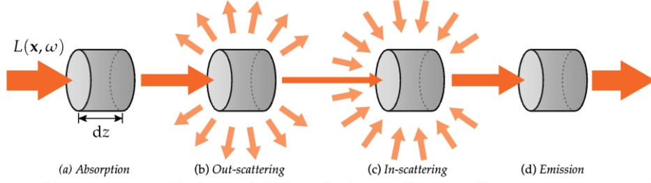
Figure 1: **Phenomenons of light modelled by Radiative Transfer Equation:** (a) Absorption, (b) Out-scattering lead to radiance loss, (c) In-scattering, (d) Emission lead to radiance gain
