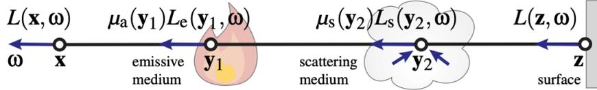
Figure 2: **Volumetric Rendering Equation:** As light travels from a surface and through a medium, it gets scattered, absorbed and emitted.  $\mu$  in the figure is same as  $\sigma$  in the text in background section.
