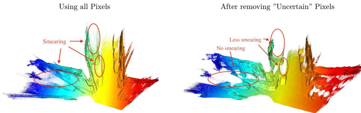
Figure 4: 3D maps created from concatenated point clouds across multiple frames of KITTI Odometry sequence 7.
